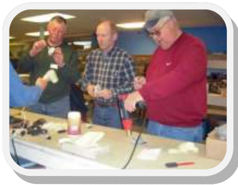
Using heat guns to dry the latex rubber, used to make rock molds.
